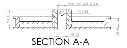
PLASTOCK ® 130T0800DFAH1S **Manufactured by Putnam Precision Molding Part Description:** www.plastock.biz .0800" Pitch (MXL) Timing Belt Pulleys For Belts up to 1/4" Wide
